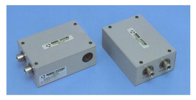
The PR-282 is an all stainless steel, 100% solid state wet/wet differential pressure transducer incorporating dual diffused piezoresistive sensing elements with stainless steel media isolation. The unit is compatible to all media encountered in HVAC applications including freon, ammonia, treated water and steam. PR-282 is designed to monitor and control pump differential pressure, CW/HW system differential pressure, chiller/boiler differential pressure drop, among other applications.
