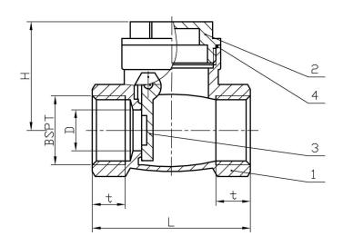
Features: The valve is designed for vertical, horizontal or angled installation for use in residential and commercial plumbing, sanitary, autoclaves, pump and
