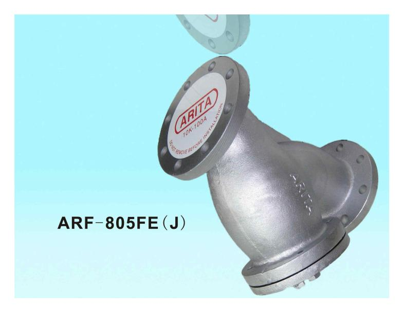
Arita Cast Iron Y-Strainer is a devices which provides a mean to remove debris from a flowing fluid in a pipeline. A perforated screen or mesh is used to trap the debris in the strainer chamber. The strainer chamber is designed with a plug or cover that can be easily removed for maintenance purposes. The Y-Strainer can be installed either in horizontal or vertical down position and must be always before the valve or equipment.
