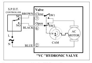
Figure 6: Actuator wiring for SPDT controller
