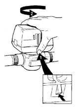
Figure 3: Actuator Head Removal.
