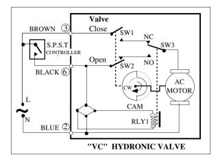
Figure 7: Actuator wiring for SPST controller
