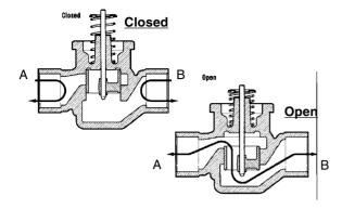
Figure 1: Fluid flow of 2-way VC series valve
